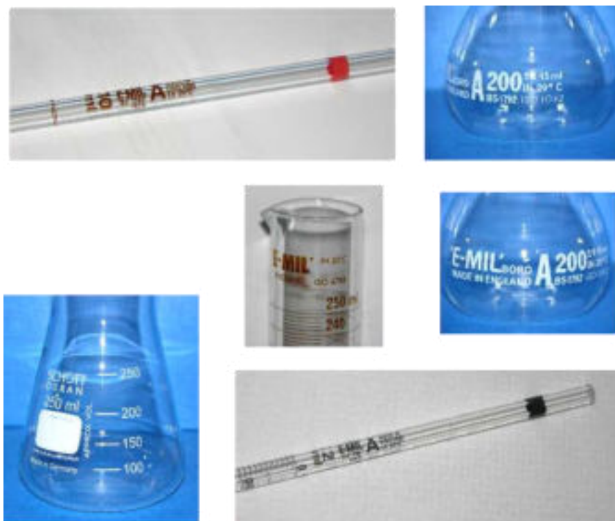
Figure 2-11. Illustrations of markings on volumetric glassware
