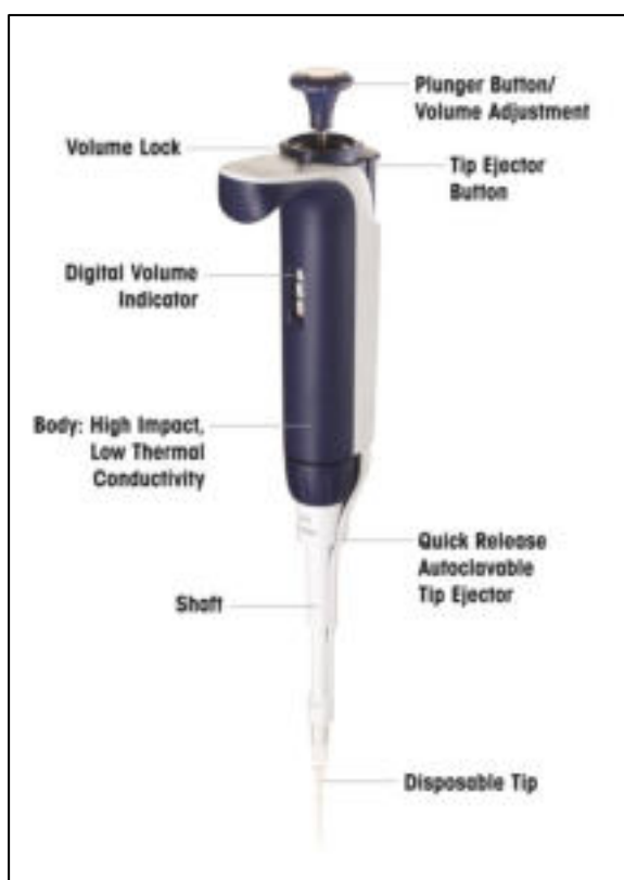
Figure 2-6. Automatic pipette components (Image courtesy of Rainin, a Mettler Toledo Company)
